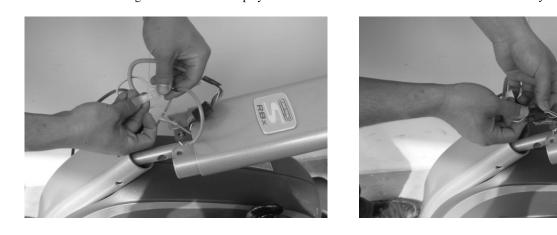
Hold the display console neck approximately three inch from the neck brackets of the bike frame. Plug the display console power, main I/O and Ground cable into their mating connectors in the display console neck. Pull coaxial cable out of console frame by white cable in handrail tube.
